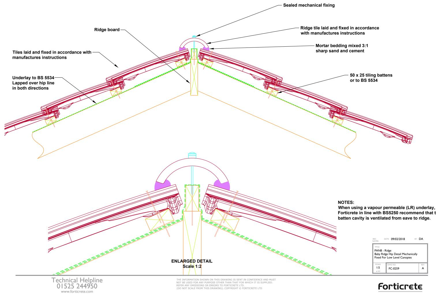
Forticrete in line with BS5250 recommend that the batten cavity is ventilated from eave to ridge.
